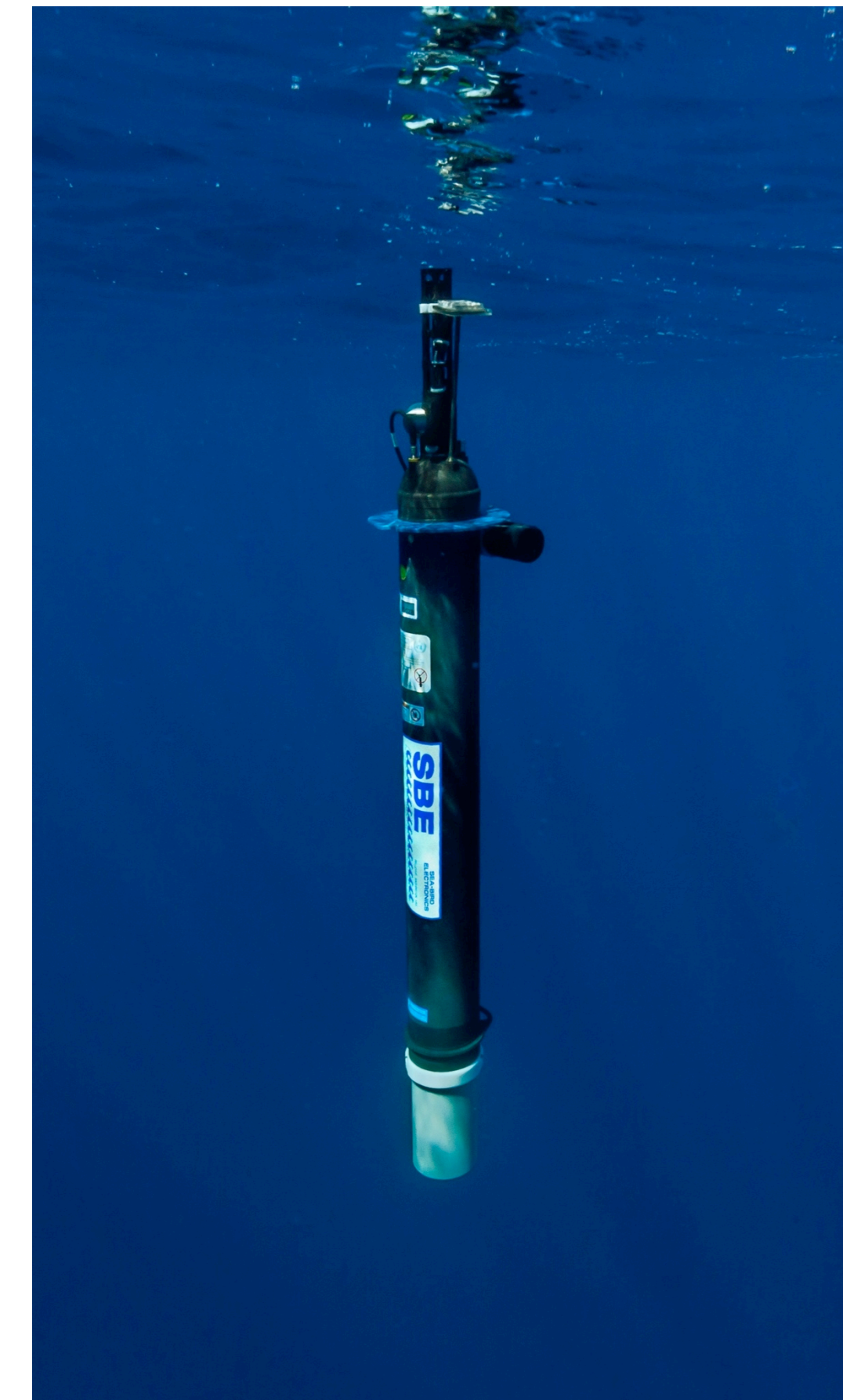
NAVIS BGC float 0028 after deployment in the Western Mediterranean. The ECO Triplet is visible on the upper right side of the float. Photo by Christoph Gerigk.
