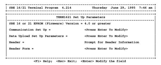
The EPROM Version is recorded on the configuration sheet of the manual and also displayed in the first line of the reply to the display status (F3) reply.
