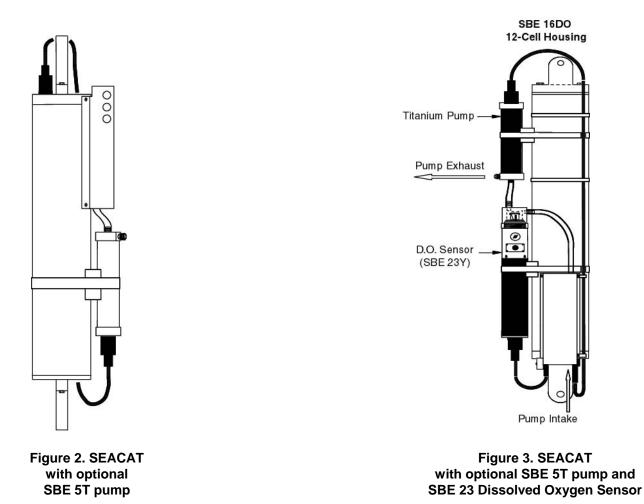
Figure 3 shows a SEACAT configured with an SBE 5T pump and SBE 23 dissolved oxygen sensor.
