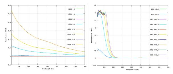
The model used to determine nitrate fits for 4 parameters: nitrate, bromide, a temperature coefficient and a linear baseline correction that accounts for all additional absorbing species. If the sample's absorption is high (default cut-off = 1.3 AU), the model can no longer be used effectively to fit parameters or determine nitrate concentration. SUNAV2 outputs a root mean square error parameter which indicates the quality of the models fit to the absorption curves.
