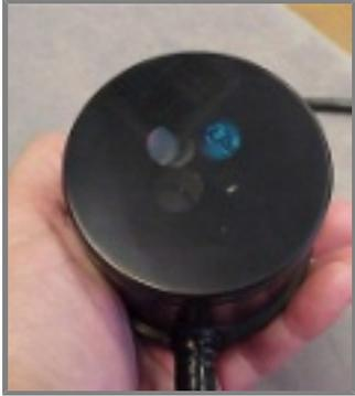
The Puck is a miniature version of the popular ECO series of sensors, specifically designed for use in AUVs, profiling floats, and Slocum gliders with a dry science bay, where space is limited and power requirements are critical.
