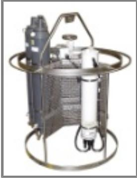
The carousel frame houses the SBE 55 system, an ideal small-boat water sampler for coastal, estuarine, and large lake ecological monitoring. The SBE 55 is light and economical and can be integrated with an SBE 19, 19plus, 19plus V2, 25, 25plus, or 49 CTD. It is available in a three- or six-bottle configuration with 4-liter sample bottles uniquely designed for the SBE 55.
